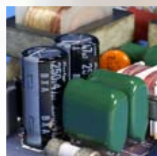
Smart ballast technology senses input voltage and automatically adjusts for 120V or 240V power.
